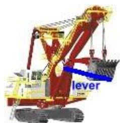
Here is another good example of a third class lever. The arm on a power shovel is a third class lever, with the fulcrum on the main boom, at the left end of the lever arm. The force is applied by the cables, somewhere along the arm.
