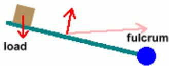
The force is applied somewhere in between by a muscle attached above the fulcrum, on the upper arm. But this force can only pull at a very small angle to your arm bone, because the muscle itself is just above the bone. It pulls, under the skin, with a force applied to your lower arm where the muscle is attached to the bone (the long arrow pointing right), but only a portion of that force (the short arrow pointing up) can be used to move the load.
